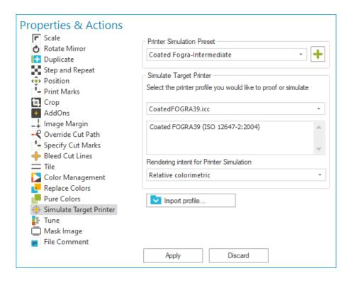
[16.1] A new centralized Image Property called Simulate Target Printer within the JobComposer allows the user to assign a proofing profile and rendering intent for image placed in the Jobs.
